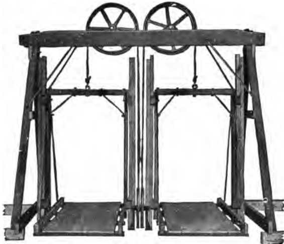
FIG. 22.—Use of a Single Pulley. Double-platform material elevator for lifting materials to a building. One elevator goes up while the other comes down, so that only force enough to lift the actual load is required.
